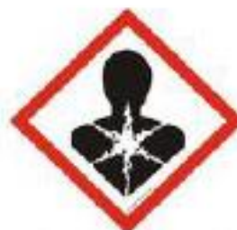
Severe health hazards
